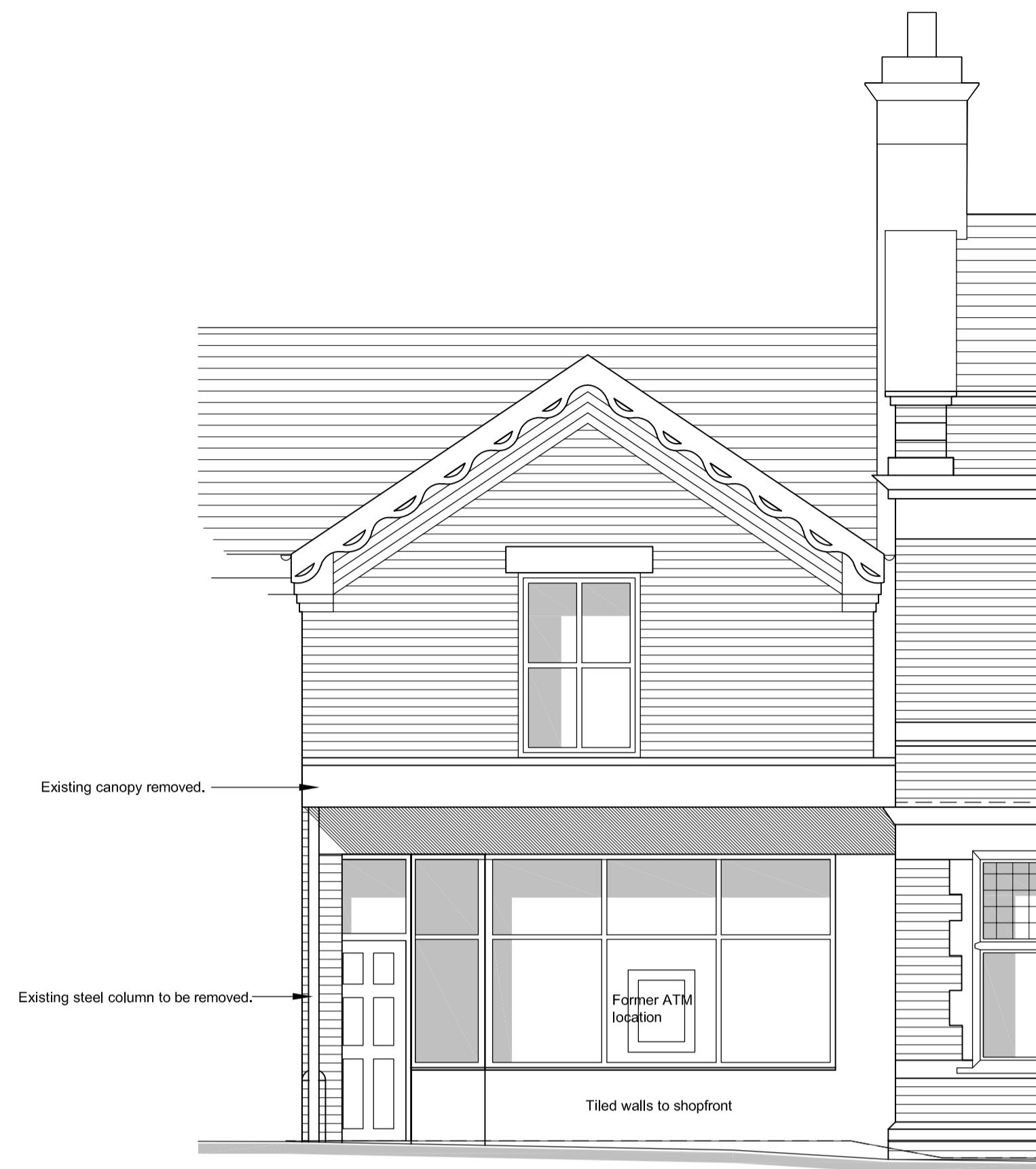
EXISTING ELEVATION (Scale 1:50)
